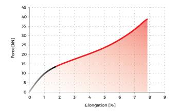
Force-elongation plot for 3DSensor core during the strength test. Limit strain: >7%.
