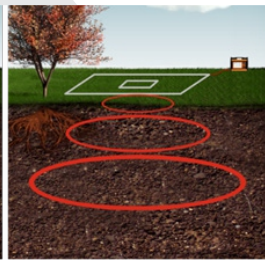
The collapsing magnetic field creates electrical currents in the ground
