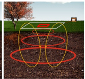
Ground currents create a secondary magnetic field recorded by the RX loop
